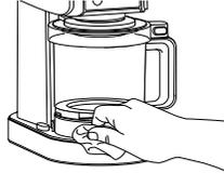
If liquid is trapped between the motor base and the platform, raise the platform to clean. Place the outer bowl onto the motor base with the handle centered below the control panel. Twist the handle to the right to raise the platform. Then use a damp cloth to clean the area between the base and the raised platform.
